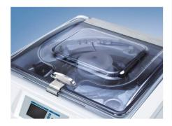
Rapid drying basin and surface of endoscope by strong air shower
